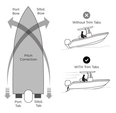
When the tabs are deployed downward, the water force on the trim tab surface creates upward pressure, raising the stern and lowering the bow. The port trim tab lowers the starboard bow, and the starboard trim tab lowers the port bow.
